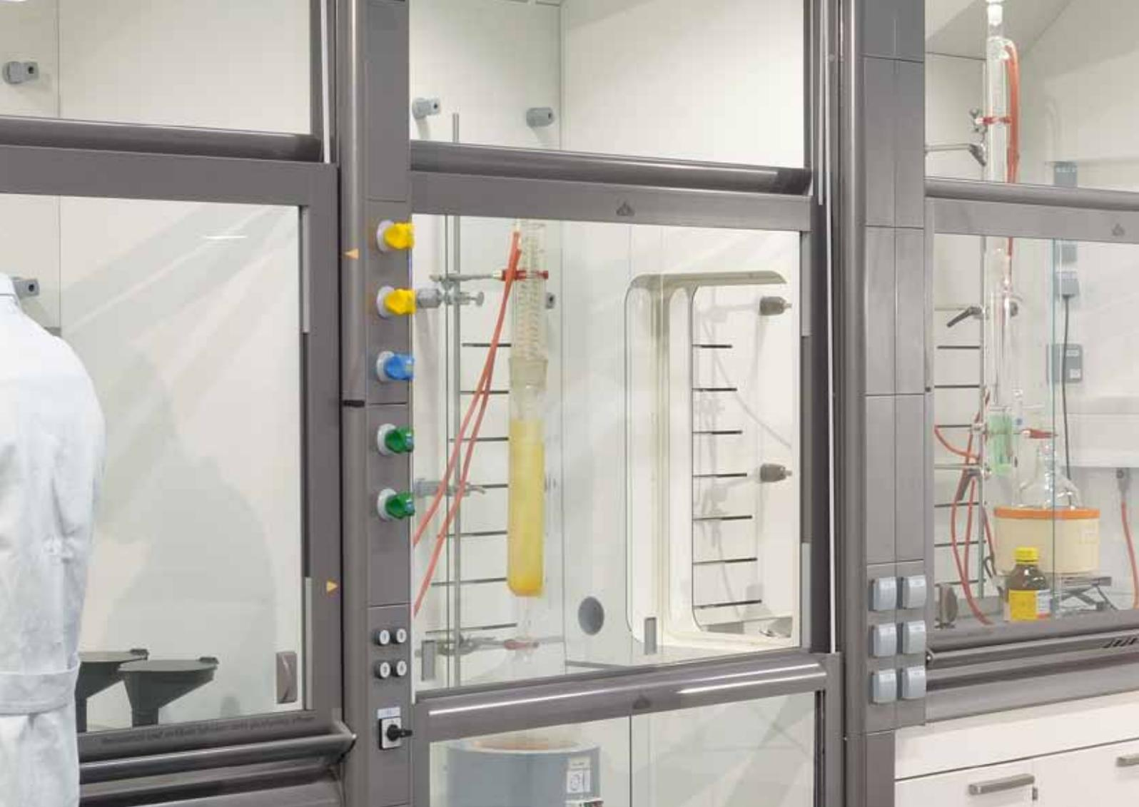
The new Secuflow offers even more safety and requires less energy. When the internal workspace is extensively equipped or a lot of movement is taking place in front of the fume cupboard, the Secuflow still shows excellent containment values – even when the sash is open. And all this is achieved with reduced extract air volumes and, as a consequence, a significantly lower energy consumption.
