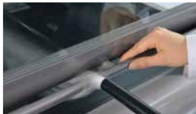
**Directs air into the fume cupboard when pushing up the sash:
